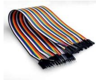
Gbr 6. Kabe Jumper
